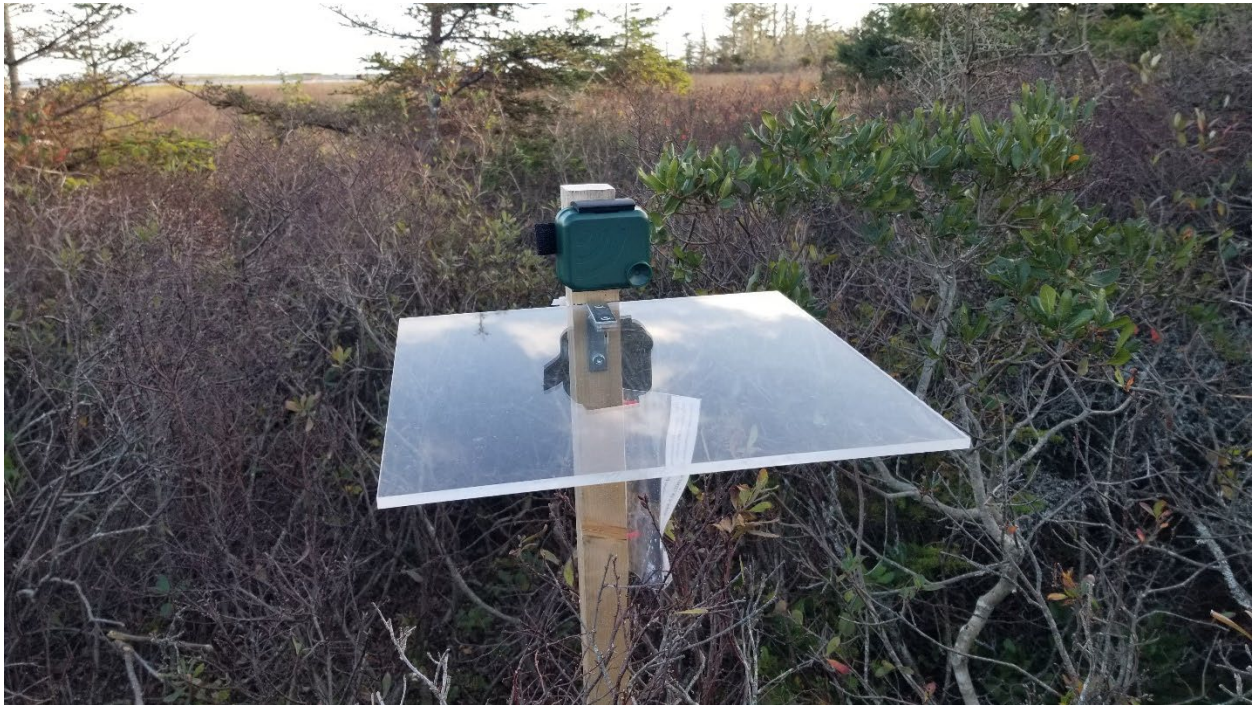
Figure 6: AudioMoth in Weather-Protective Case over Plexiglass Plate (Photo by Alix d'Entremont)
