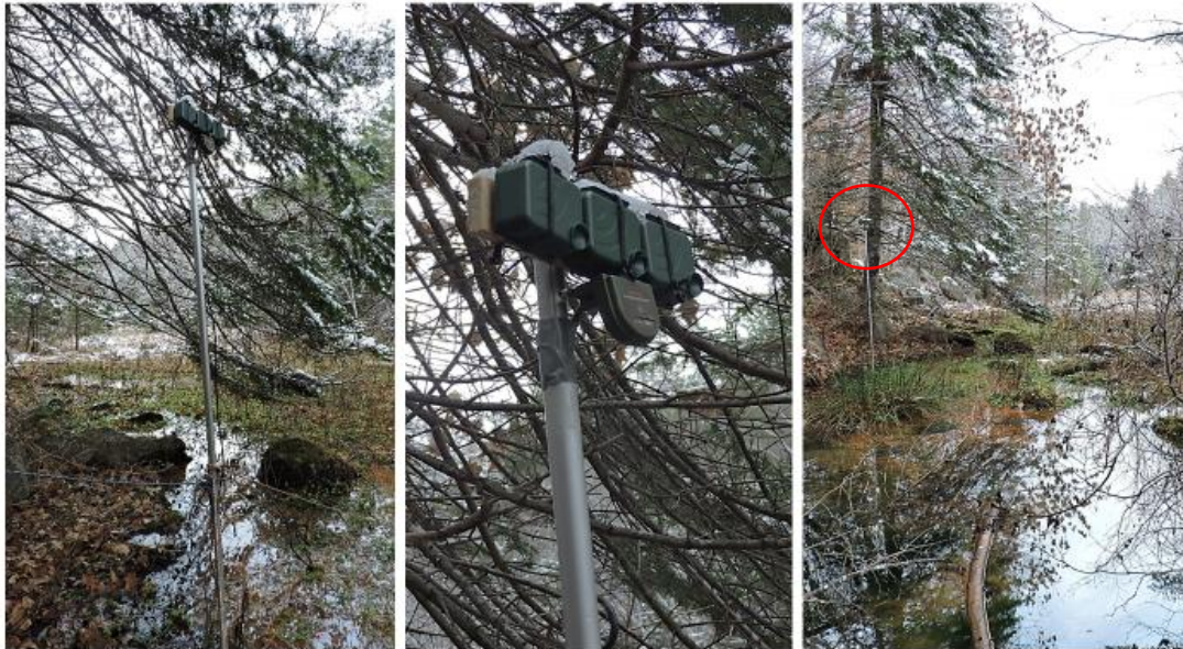
Figure 2. Bat overwintering site acoustically sampled during December 2020 using 3 Audiomoths and 1 Song Meter SM4BAT-FS with a U2 Ultrasonic Microphone. Acoustic equipment was positioned outside ~11 away from the entrance to the site.
