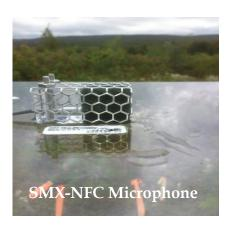
Wildlife Acoustics also produces a night flight call microphone, the SMX-NFC, to be used with the Song Meter. This weather-resistant microphone rests on a flat horizontal plate creating a pressure zone resulting in a 3-6 dB gain within a beam angle of 125 degrees.
